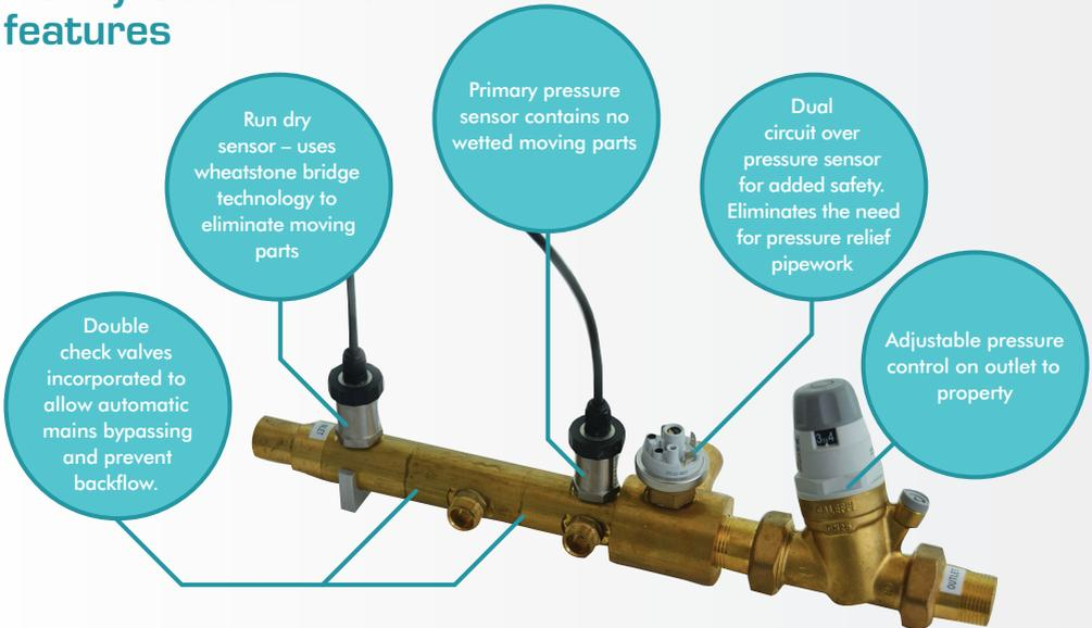
**Dual circuitry** The system controller incorporates a number of safety features. As well as the primary pressure sensor there are two other sensors. These provide **RUN DRY PROTECTION** and **OVER PRESSURE PROTECTION**.
